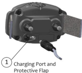
Lift the protective flap over the charging port (1) and insert the charger.
